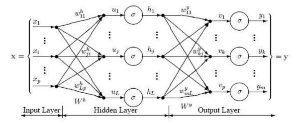
Fig: 3. A perceptron network with three layers
